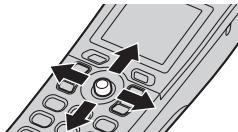
It can also be used to select the center soft key icon, by pressing down on the center of the joystick.
